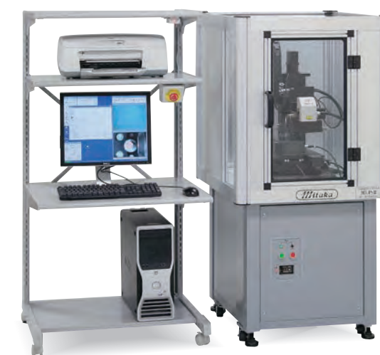
Model: MLP-2 (360-degree measurement model) Measuring range: XYZ = 120mm X 90mm X 130mm AF (R) = 40mm, AZ (θ) = 360° Scale resolution: XYZ = 0.1μm, 0.1μm, 0.1μm AF (R) = 0.01μm, AZ (θ) = 0.001° Applications: precision gears, endmills, punches, molds for connectors, etc.
